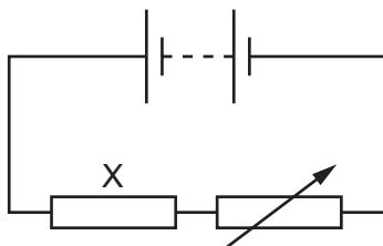
The power dissipated in resistor X is 7.2 W when a current of 3.0 A passes through it.
