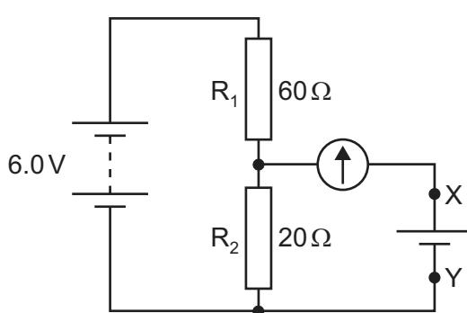
The circuit is to be used to test whether the electromotive force (e.m.f.) of a particular cell is  $1.5\text{V}$ . The cell is connected between terminals X and Y in parallel with  $R_2$  and in series with a galvanometer.
